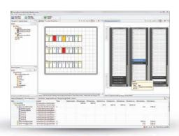
Instant overview of data center operations through inventory management, PUE calculator, real-time device alarms, and location-based drill-down
